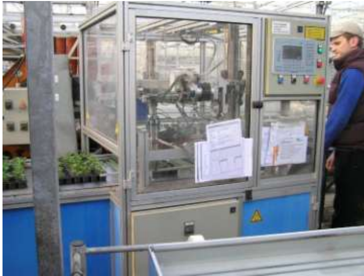
Figure 34 Robot Transplanter for Containerised Plants
